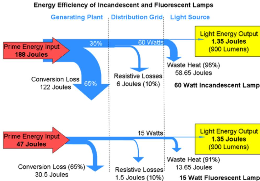
For comparison, a compact fluorescent lamp (CFL) produces between 50 and 60 lumens per Watt. By using fluorescent rather than incandescent lamps, the power consumption of the lamps can be reduced from 60 Watts to 15 Watts for the same light output. The consumer saves a modest 45 Joules per second but the corresponding prime energy consumption is reduced by a massive 141 Joules per second.
